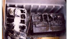
Batteries, like these conversional wet-cells, have always had the potential to start fires due to their high energy content. These caught fire when an errant wrench contacted both terminals (Claim #0205712). Newer technology batteries with higher capacities and less forgiving charging characteristics will require even more caution along with sophisticated monitoring.
